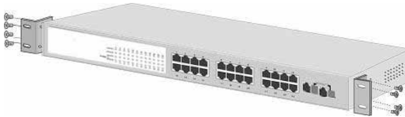
Figure 2-4 Attaching the brackets to the Web Smart Switch
